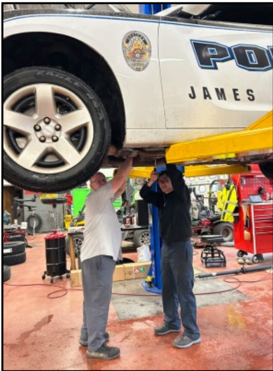
Brock Bealer, WJCC student, Automotive Intern, replacing an engine oil cooler and driveshaft.
