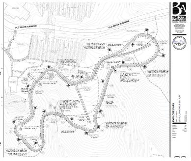
The trail was constructed over six weeks from September to October. It is a 6-foot wide packed, stone dust surface trail with grades of 8% or less throughout, able to accommodate wheelchairs or individuals with limited mobility. Construction included the electrical infrastructure to handle the event, such as six new panel boxes. The trail was completed on schedule at the cost of \$169,502.42.
