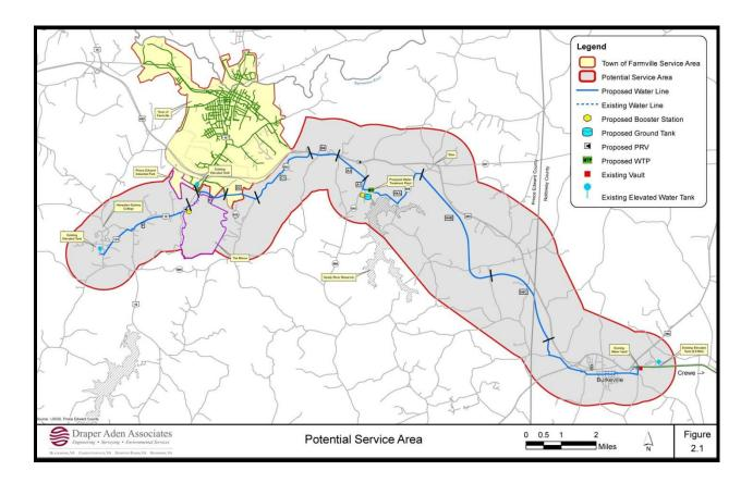
The eastern water system will follow a power line until Route 605, and then head north to provide availability to the Rice community, and then will follow the High Bridge Trail to Nottoway County to connect to the existing water systems in Burkeville and Crewe. There are two locations off the High Bridge Trail where water could be extended to serve areas along Route 460.
