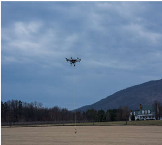
DJI Matrice 600 Aircraft Showing Payload Drop Capability
