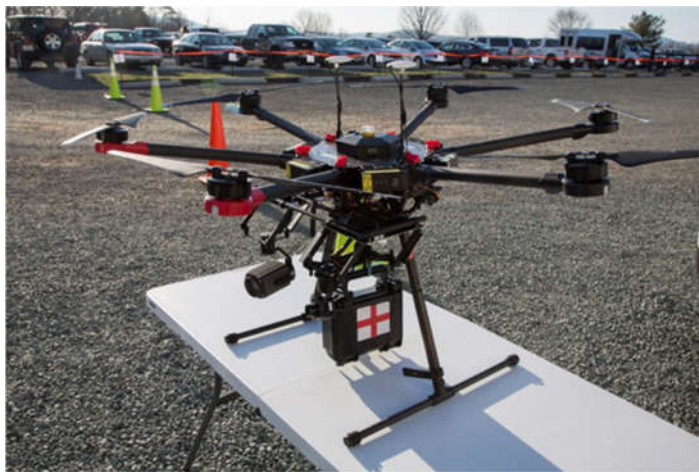
DJI Matrice 600 Aircraft with High Powered Camera, FLIR and Medication Payload
