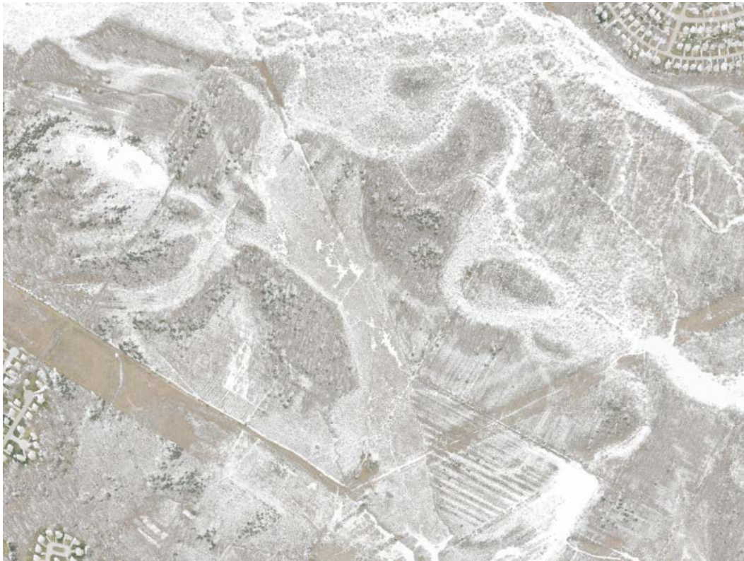
Figure 2: Same imagery as before, with infrared band exposed. The closer the white dots are to one another, the higher the moisture content. With solid white representing water.
