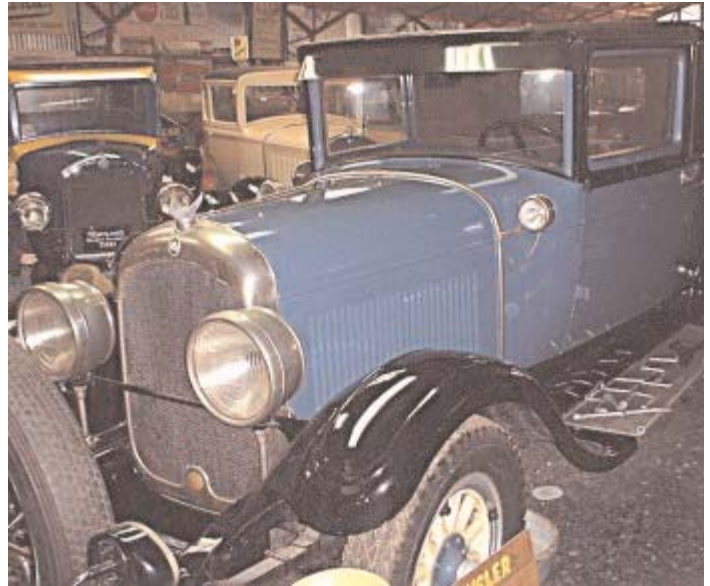
This 1928 Chrysler 72 features a rumble seat body style produced by Fisher Body. It also has a Red Head high compression engine.
