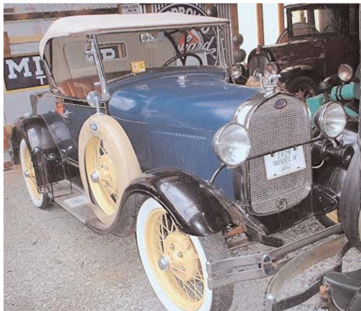
This 1929 Ford Model "A" has a DeLuxe Rumble Seat body style and overhead valves as well as a hemi-type head. It gets 20 miles to the gallon.
